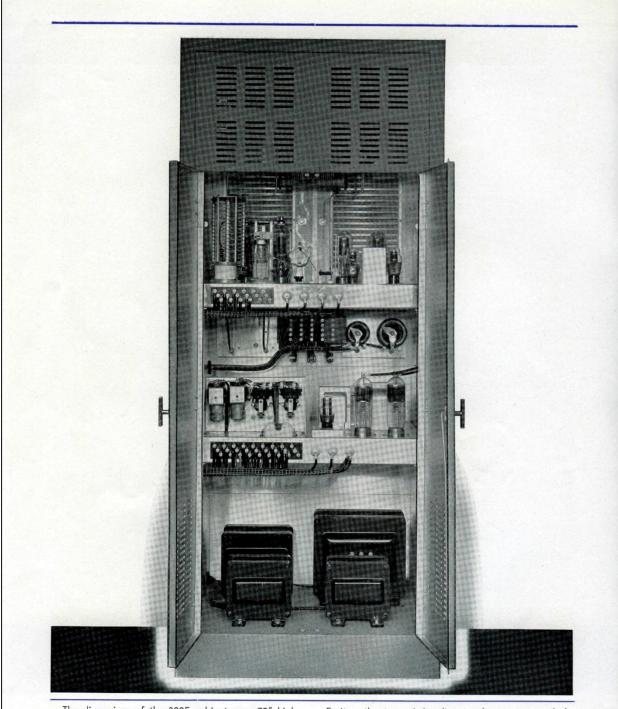
The dimensions of the 300F cabinet are—72" high, 30" wide and 24" deep. The sides of the cabinet are removable and expose the internal cabling and provide space for the incoming leads. Installation of the transmitter consists merely of connecting the power leads, the audio input leads, the transmission line to the 40C
