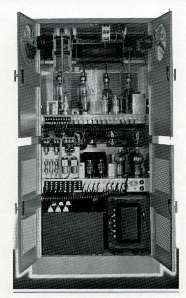
power interlocks as a safety measure, and the upper rear doors carry the blowers which assure proper ventilation.
