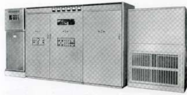
240D-2 UHF 10 KW PAs – 400–550 Mhz Relay Commands to Capsule – 2 per Ship Rose Knot Victor – Costal Sentry Quebec
